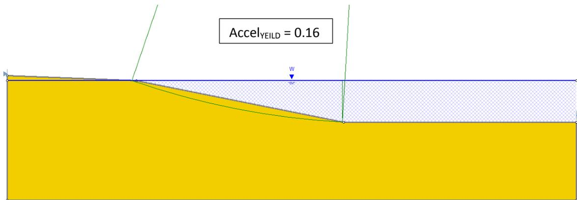
Based on the results above, the proposed slopes at the design grades indicated have a higher yield acceleration compared to the calculated peak ground accelerations at the site indicating that slope failure due to seismic forces is not expected.
