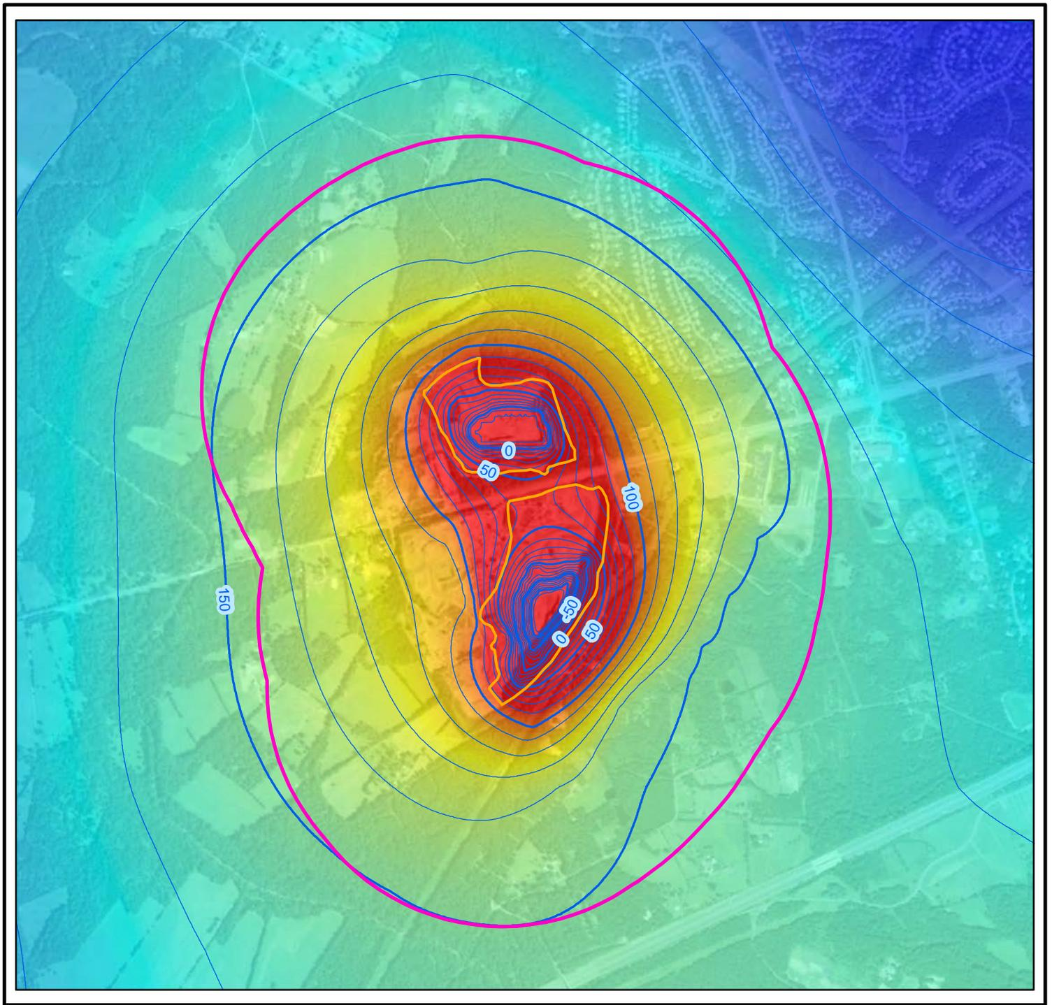
**Figure 4a: Model-Predicted Groundwater Elevations at Fill Sequence 1**
