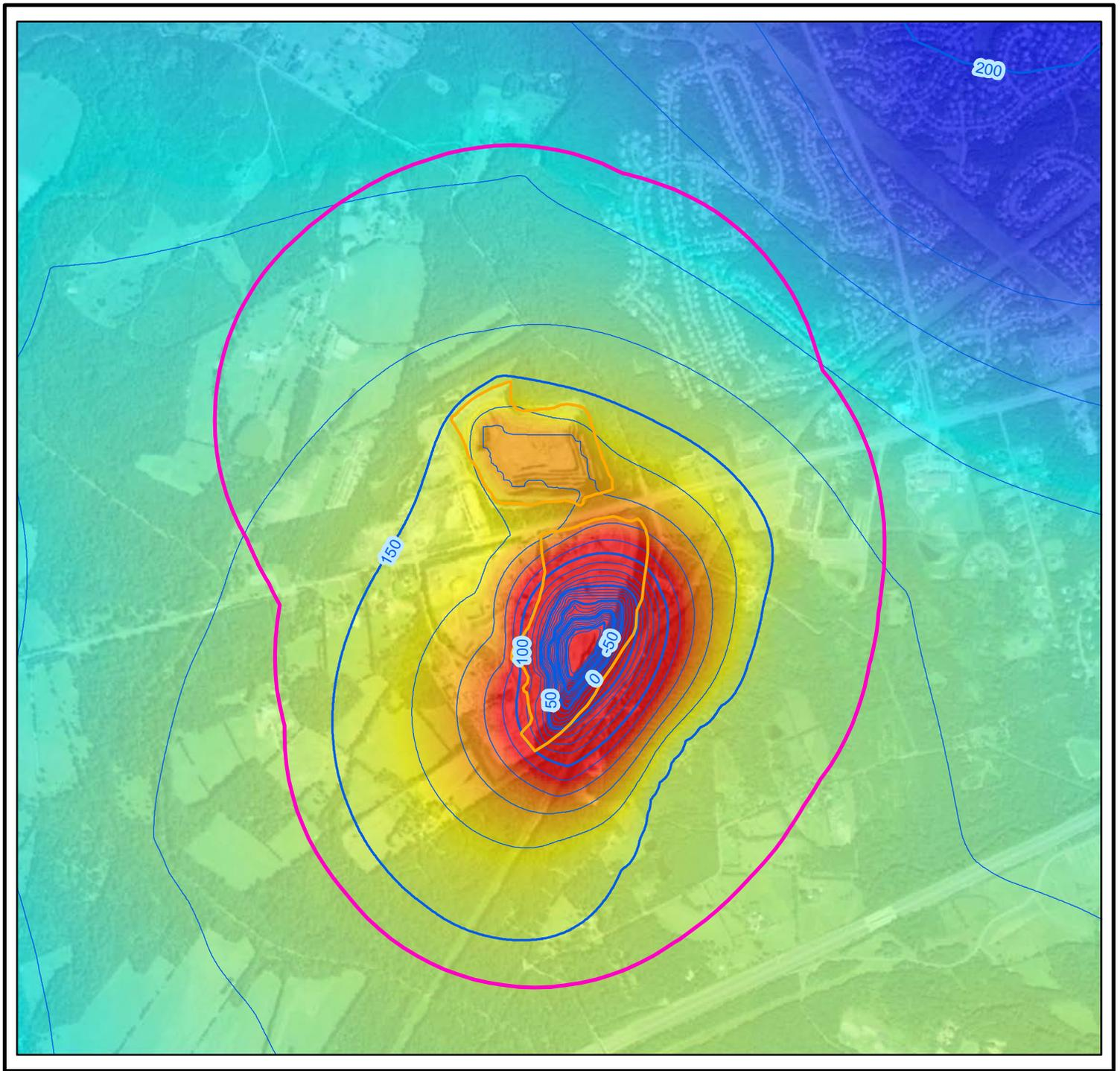
**Figure 4e: Model-Predicted Groundwater Elevations at Fill Sequence 3**
