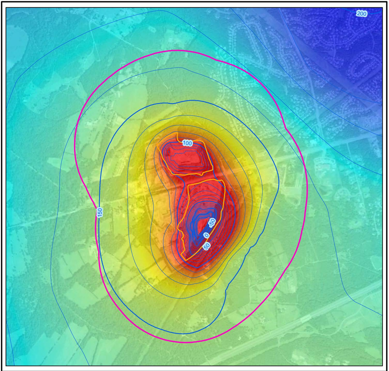
**Figure 4c: Model-Predicted Groundwater Elevations at Fill Sequence 2**
