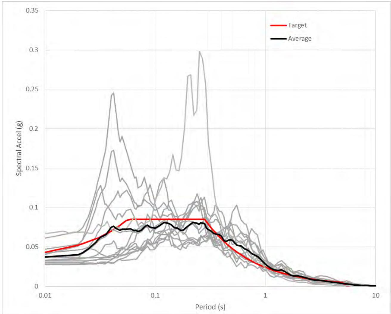
The selected ground motions were evaluated in DEEPSOIL v7.0 software for site response using the equivalent linear method. Assumed soil properties were selected for the fill in the quarry. These properties are considered appropriate for the materials in the general region that are most likely to contribute to the fill placement. Below are plots summarizing the soil properties.
