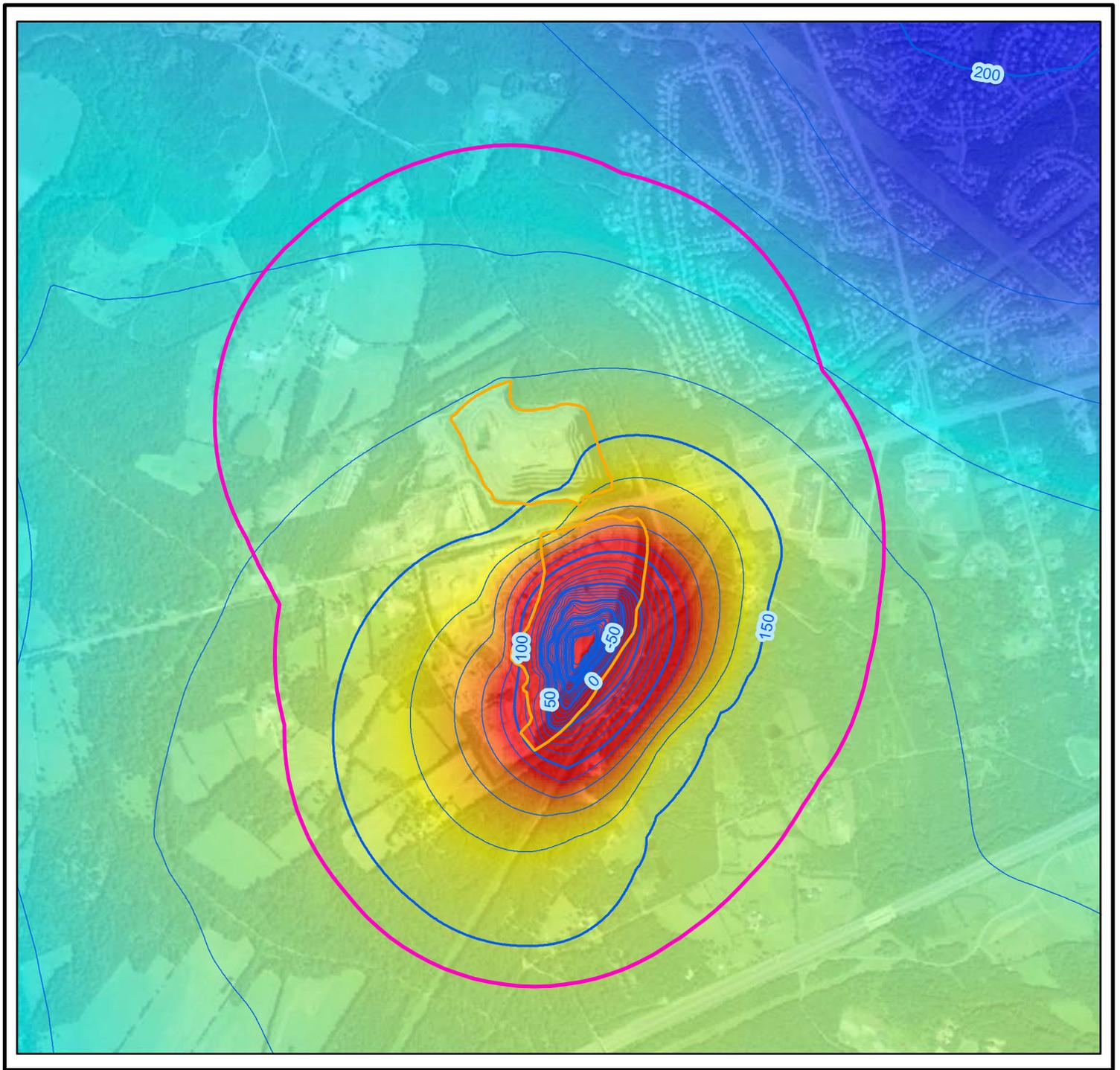
**Figure 4g: Model-Predicted Groundwater Elevations at Fill Sequence 4**
