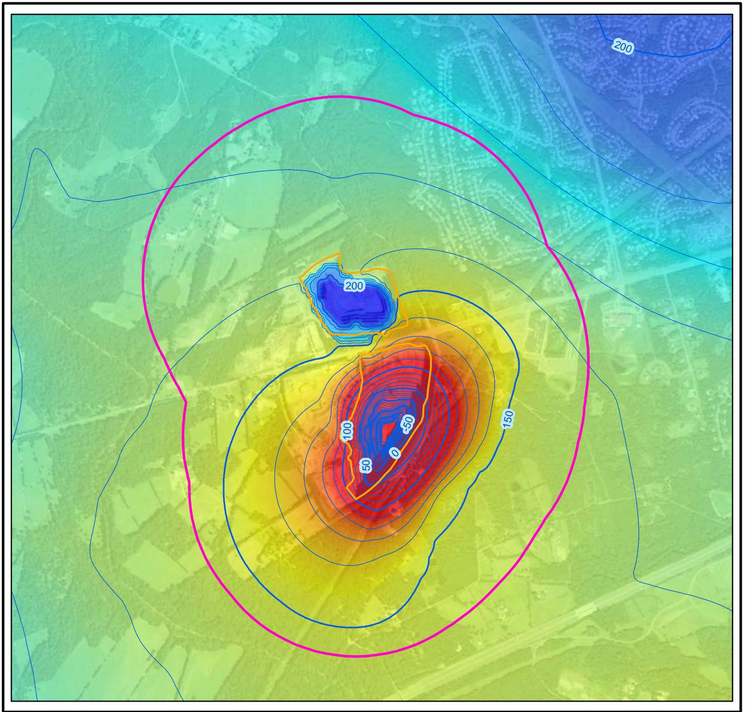
**Figure 4i: Model-Predicted Groundwater Elevations at Fill Sequence 5**
