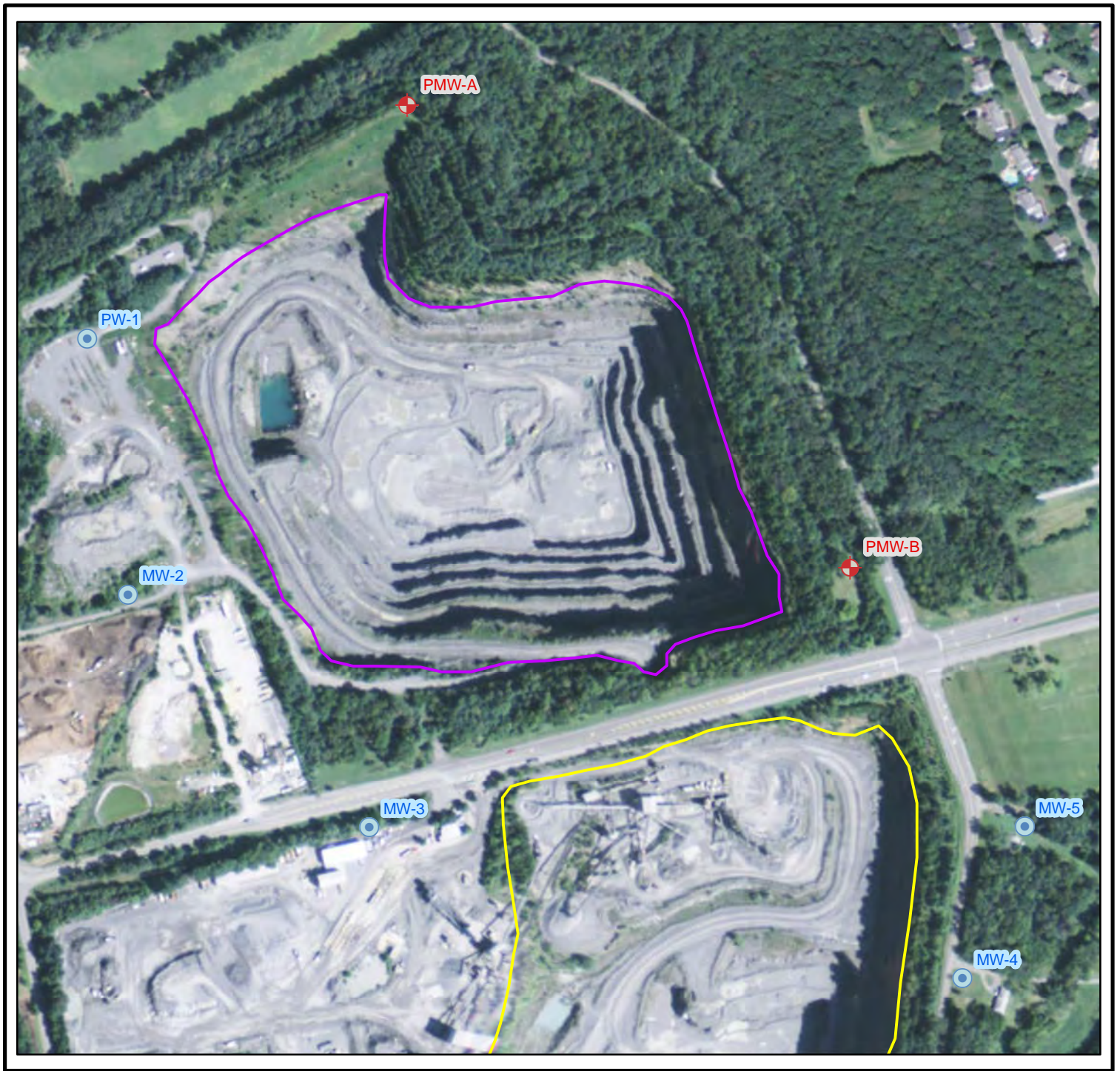
Figure 2: Proposed Bedrock Monitoring Wells
